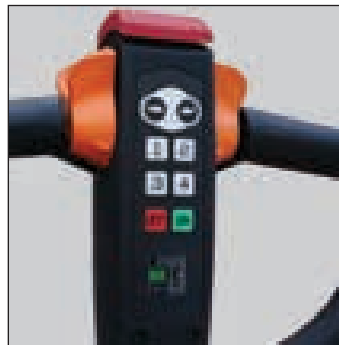
Turtle speed setting reduces drive speed by 50% for precise positioning.
